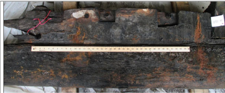
Figure 47. Transom stern construction.
