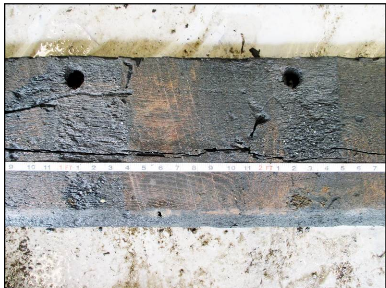
Figure 54. Inner face of garboard strake. (Note: the rabbet bevel, pit saw marks, and wear patterns where the strake would have been attached to floors.)
