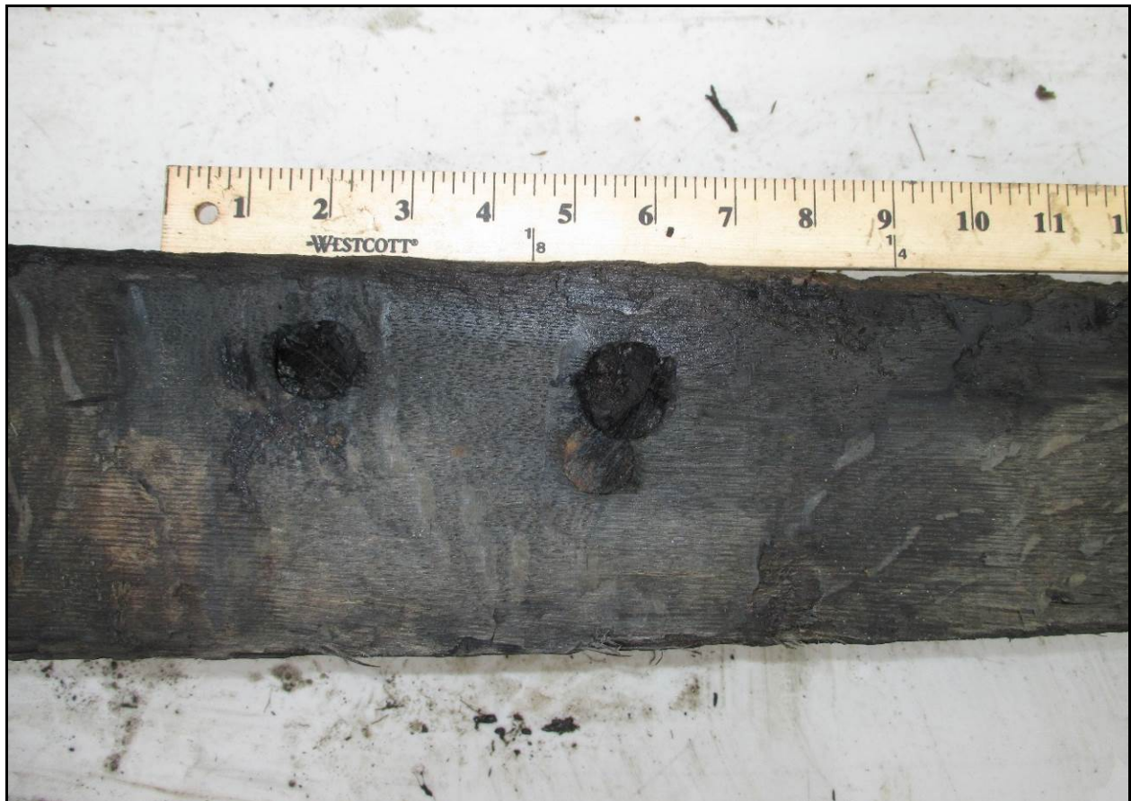
Figure 83. Example of refastening (center of photo).
