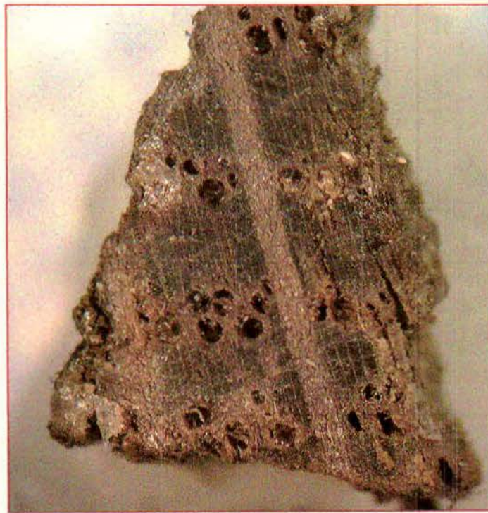
Figure 1: White oak structure is clearly evident under magnification. (Keelson).
